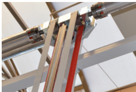
Bystronic glass gripper beam held by BRECOmove timing belts
